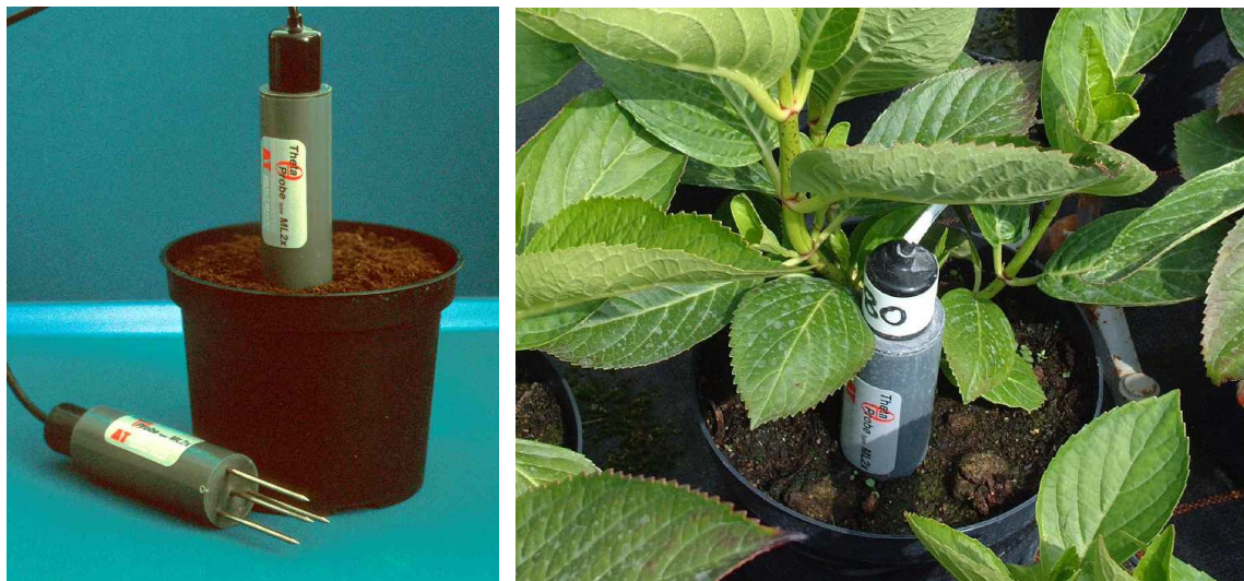
Figure 4.5 The ThetaProbe on the bench, pushed into the surface of an empty pot and partially buried in a Hydrangea pot to monitor and control water content at mid-depth (35 - 95 mm).
