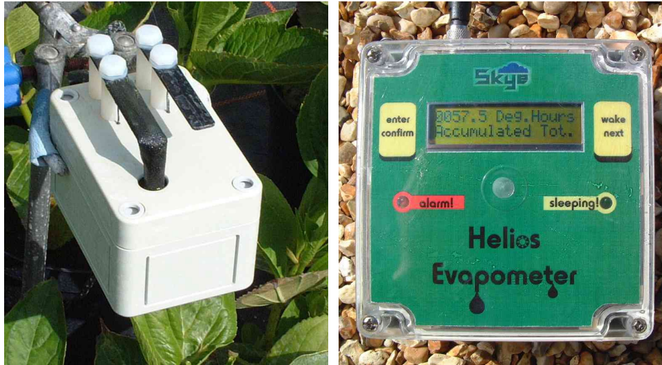
Figure 4.4 The evaposensor (left) and the EvapoMeter used to integrate and display its readings (right).
